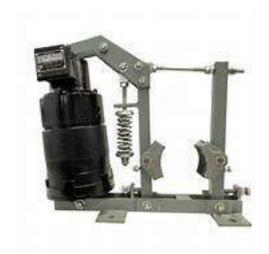
A thruster brake is a type of braking system commonly used in industrial applications to control the speed and stop the motion of hoists, cranes, winches, and other similar machinery. It is an electro-hydraulic braking system that utilizes a device called a thruster, which generates the braking force.
